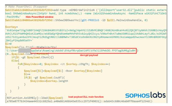
The reflectively loaded payload is the Solarmarker backdoor.
