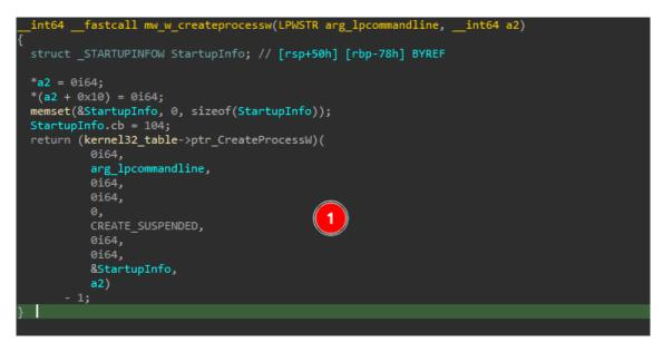
Figure(21): create a suspended process
