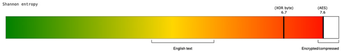
Fig. 4 - Shannon entropy of similar responses from C2 server, encrypted through different methods.
