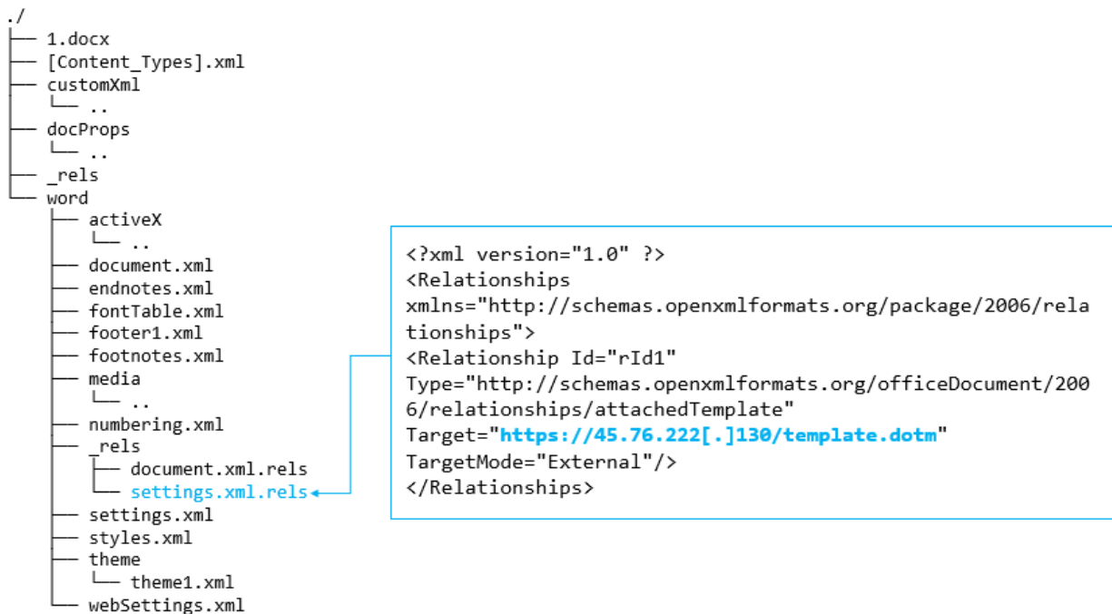
Figure 4. Word file's structure that uses Remote Template Injection
