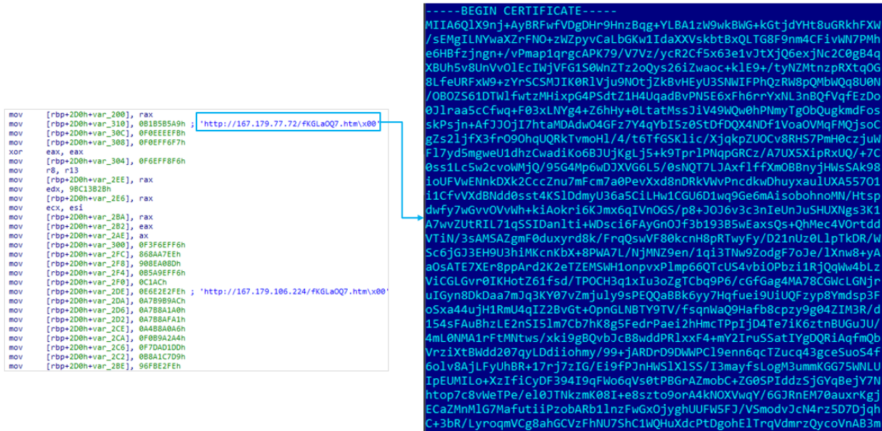
Figure 12. C2 server information and the Fake PEM file embedded in the Downloader Shellcode
