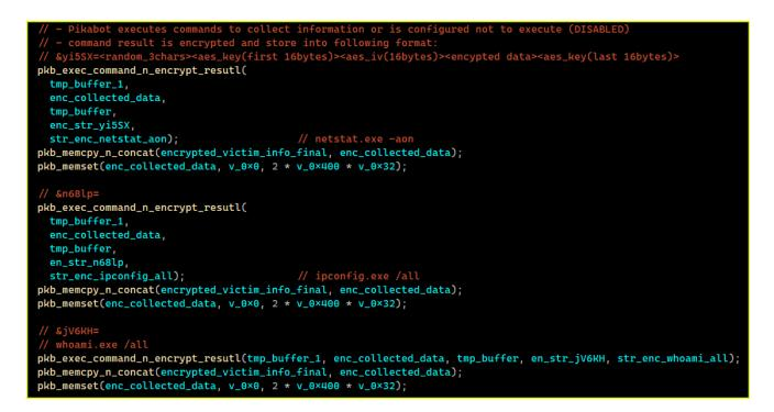
The results of these commands are also encrypted and stored in the same way as above. However, the sample that I am analyzing is configured as **DISABLED**.
