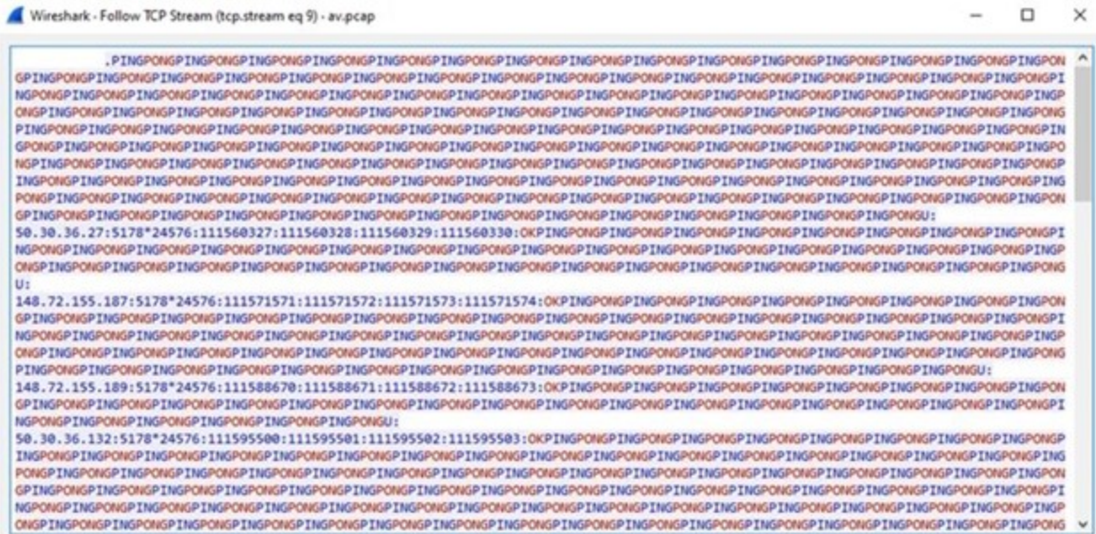
Figure 2: Example of the PING/PONG traffic
