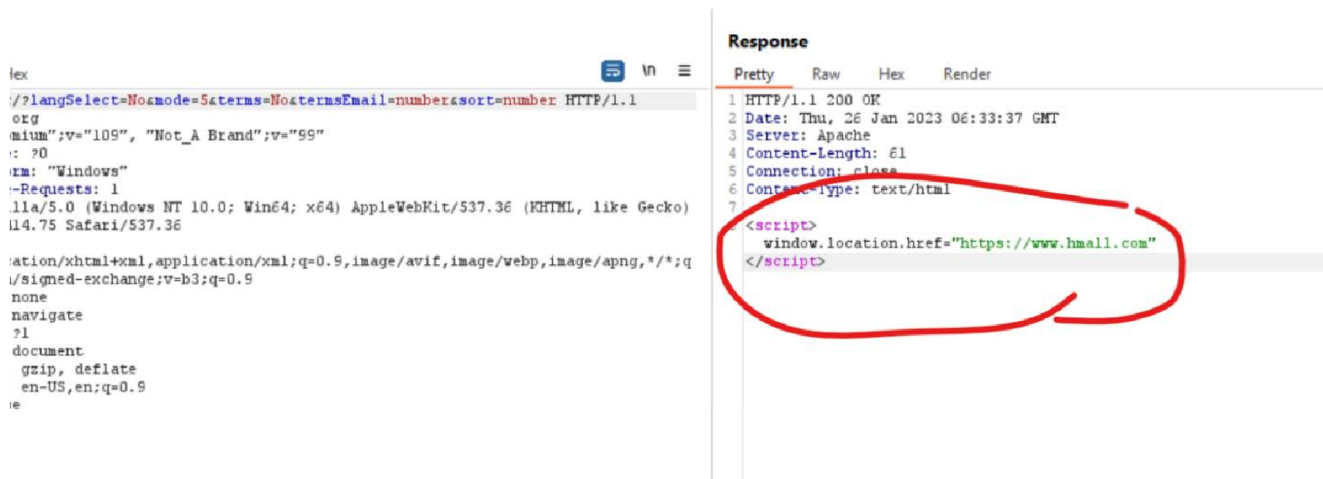
Figure 5 Example of redirection from the phishing kit when validation checks aren't valid
