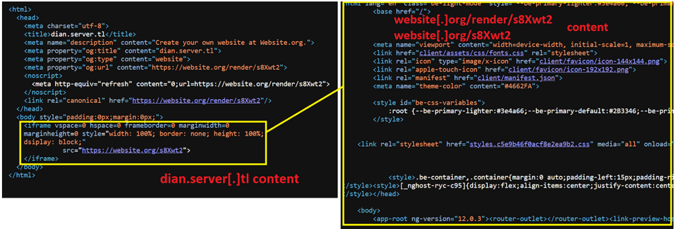
Figure 4: The content the victim sees is shown on the left, which is loaded from the resource shown on the right
