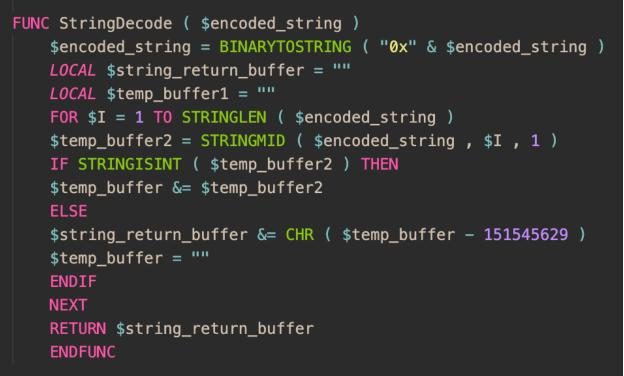
New decoding function (function and variable names renamed for clarity)
