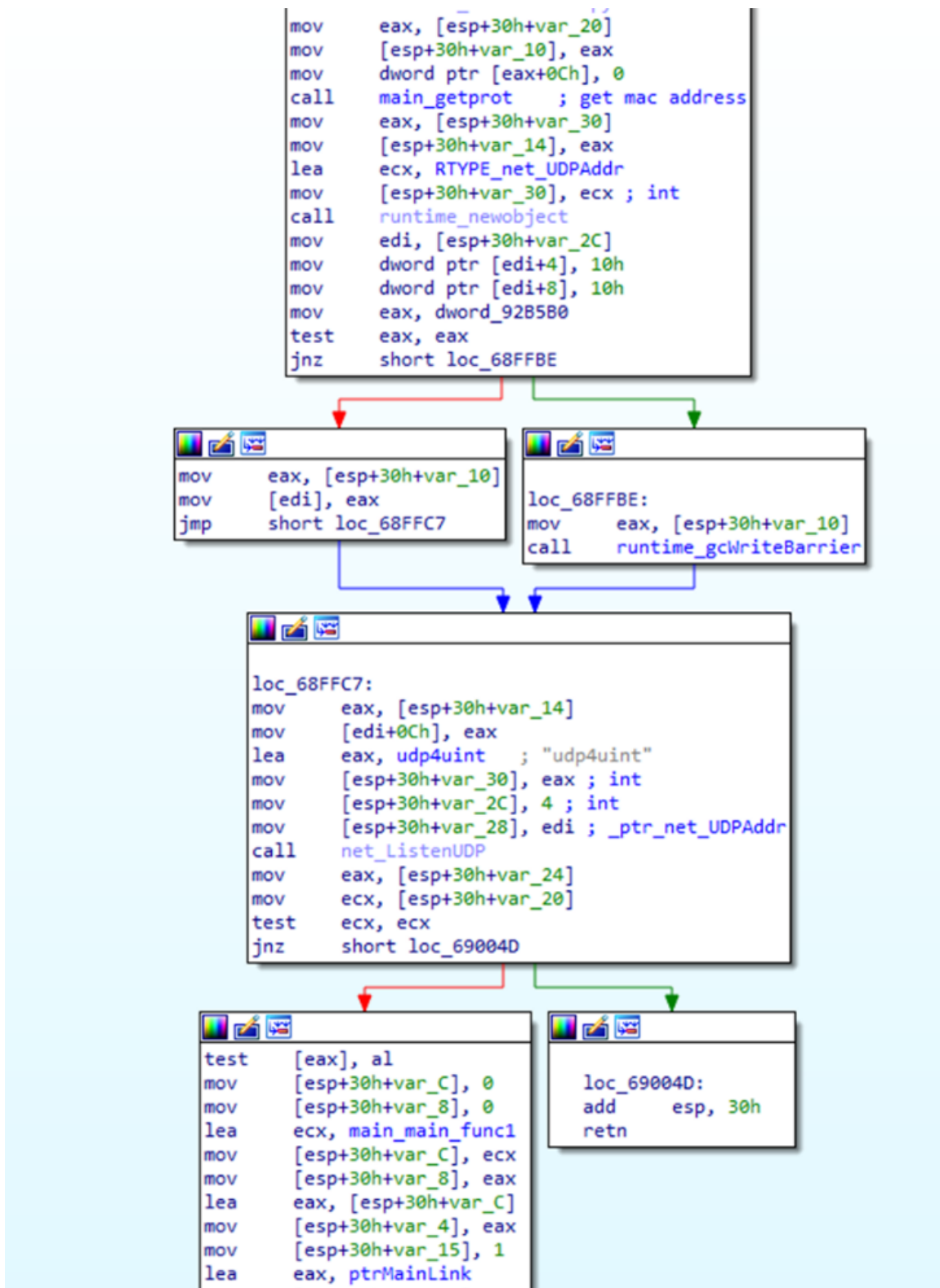
Figure 2: Method that generates the host port to bind to in a Windows device
