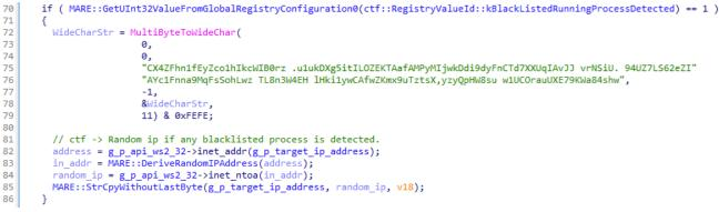
QBOT using randomly generated IP address if fuse is set
