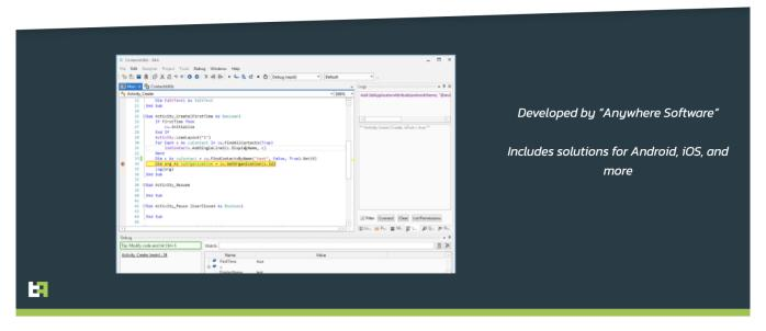
B4A belongs to the **B4X suite**, developed by "Anywhere Software". Its name comes from its similarity to BASIC, despite it being an independent and proprietary language in its own. The framework relies on a combination of simple UI based designer tools and its BASIC-like language. The framework will then interpret the designs and code in the project and will create a corresponding, valid APK.
