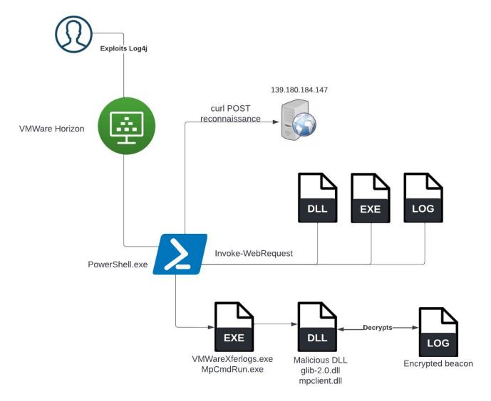
Once the attackers gained initial access via the Log4j vulnerability, reconnaissance began using <u>PowerShell</u> to execute commands and exfiltrate the command output via a POST base64 encoded request to an IP. Examples of the reconnaissance activity can be seen below:
