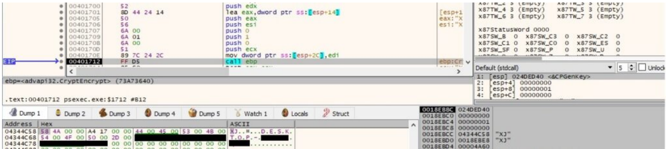
Figure 63 The encrypted buffer size and the encrypted buffer are written to the “\\192.168.164.130\pipe\PSEXESVC” pipe:
