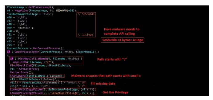
If the file name can't be obtained, the c letter is used by default (it's the expected one). If the sample has a different name, then some bytes of the string get placed somewhere unexpected on the stack, almost certainly leading to a crash later on.
