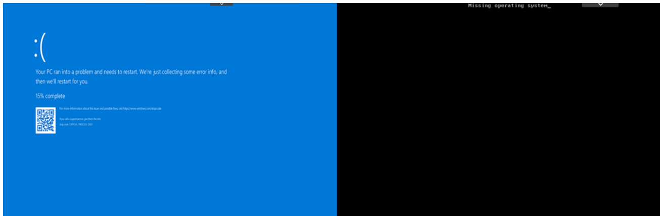
Figure 8. Once the deletion of data is complete, a reboot executes, and the system is no longer operable
