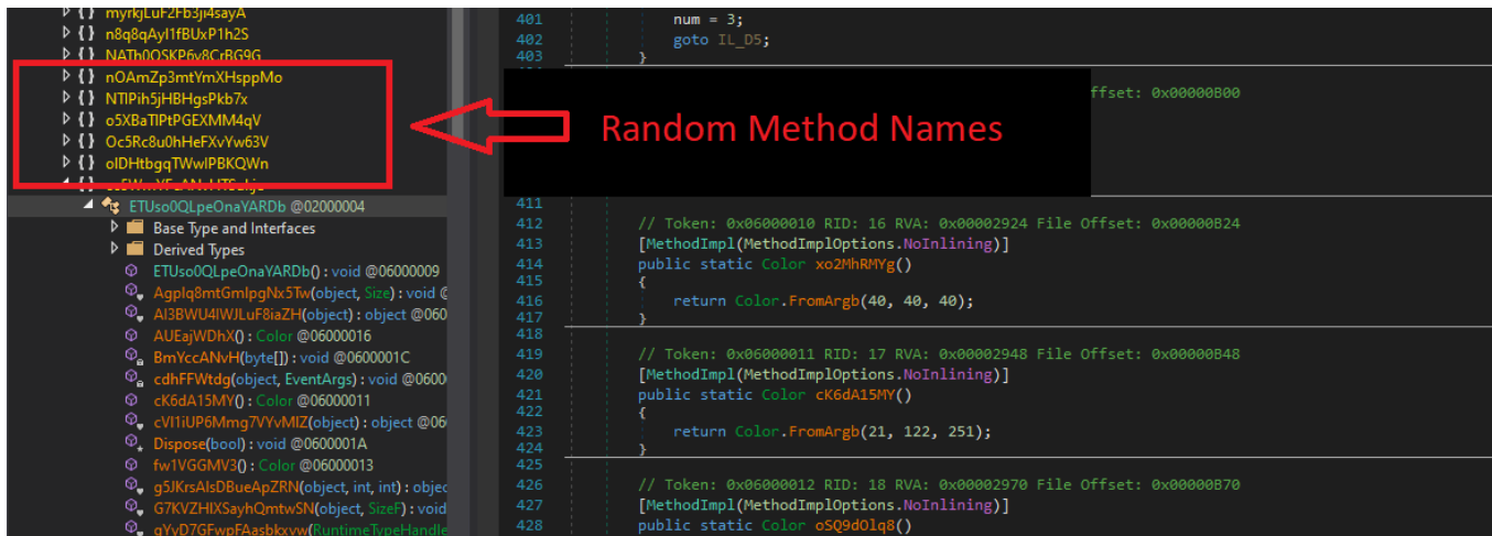
Fig.1 Main Payload Obfuscation
