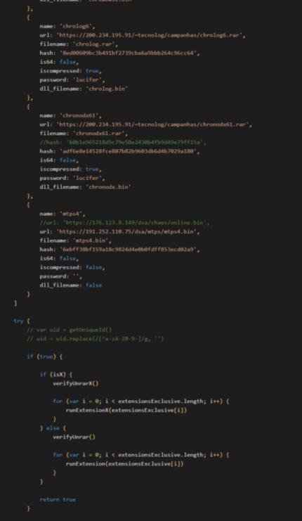
The extensions are separated into password-protected archives vs encrypted binaries. The non-compressed payloads are PE files that can be run independently while compressed ones add necessary NodeJS packages for the extension to run. Below is the example of chremows63\_64 archive contents:
