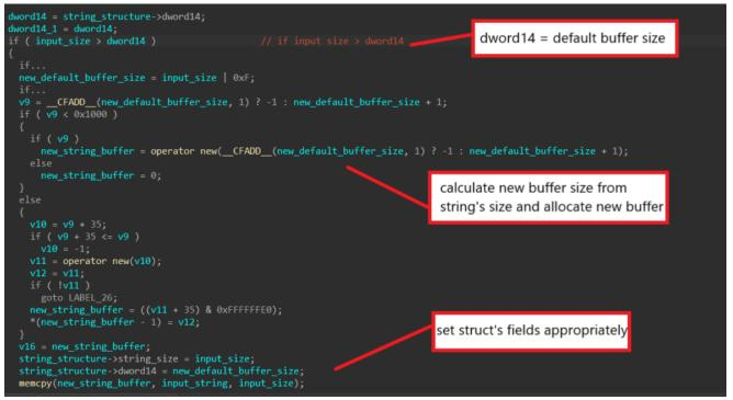
In this part of the function, the field's value is compared to the string's size, and if it's smaller, the malware will allocate a new buffer that is one byte bigger than the string's size. This new size is set back to the *dword14* field, and the newly allocated buffer is later set to the **pvoid0** field and has the string input written to it. From this, we can assume the *dword14* field contains the default buffer size for the structure's string buffer.
