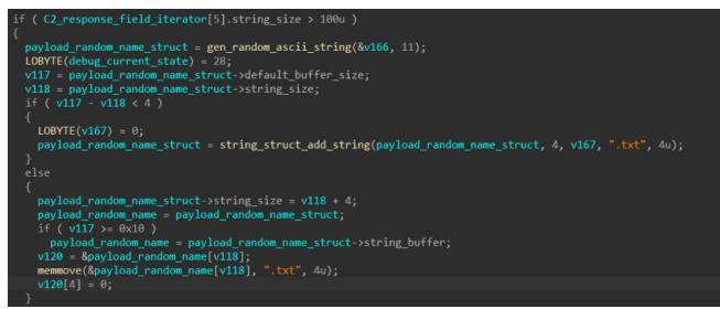
The malware then calls **std::\_Fiopen** with the newly generated filename to get a file stream to write to. It extracts the content of the executable from the response field and writes it to the file stream.
