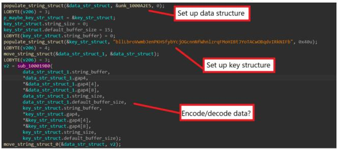
Upon analyzing **sub\_100019B0**, we can see that the algorithm boils down to a single for loop. First, SQUIRRELWAFFLE allocates an empty string structure to contain the result of the algorithm. Then, the malware uses a *for* loop to iterate through each character in the data, XOR-ing it with a character from the key.
