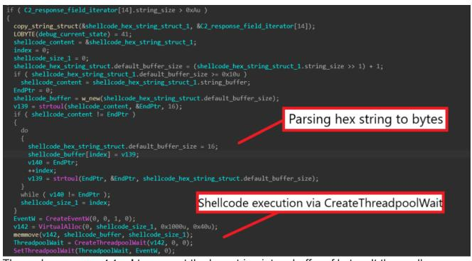
The malware uses **strtoul** to convert the hex string into a buffer of bytes. It then calls **CreateEventW** to create an event object, allocates virtual memory, and writes the buffer into the allocated memory.
