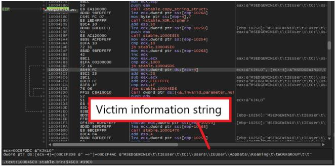
Since this victim information string is later delivered to C2 servers, SQUIRRELWAFFLE encodes it using the XOR cipher with the key "KJKLO" and Base64 to avoid sending it in plaintext.
