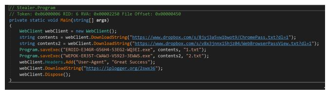
The tools are obfuscated in the same manner as described in the previous section. The output is exfiltrated to an attacker-controlled server different from the C2. Once the upload is performed, both results and the utilities are removed from the system.
