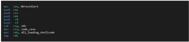
Figure 6. Malicious payload overwriting the original NtTestAlert() routine
