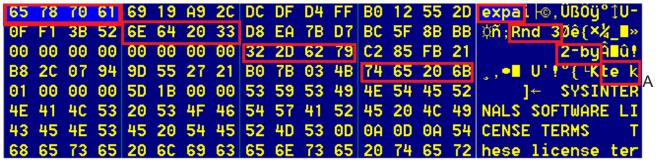
partially encrypted file example showing how Salsa20 "steps" through a file (note the position of "expand 32-byte k")
