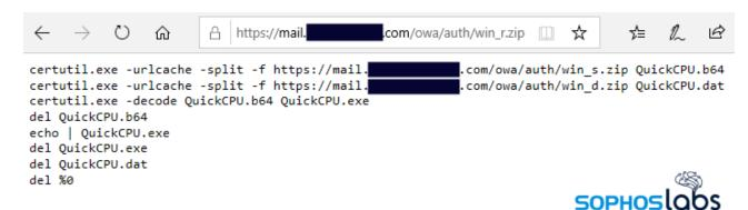
The first file is written out to the filesystem as QuickCPU.b64. The certutil application is designed to be able to decode base64-encoded security certificates, so the attackers have leveraged that functionality by encoding an executable payload in base64 and wrapping it in headers that indicate it is some form of digital certificate.
