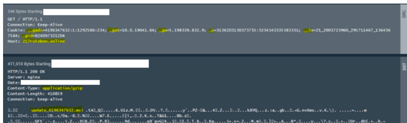
Figure 4: PCAP of Traffic to Suspect Domain
