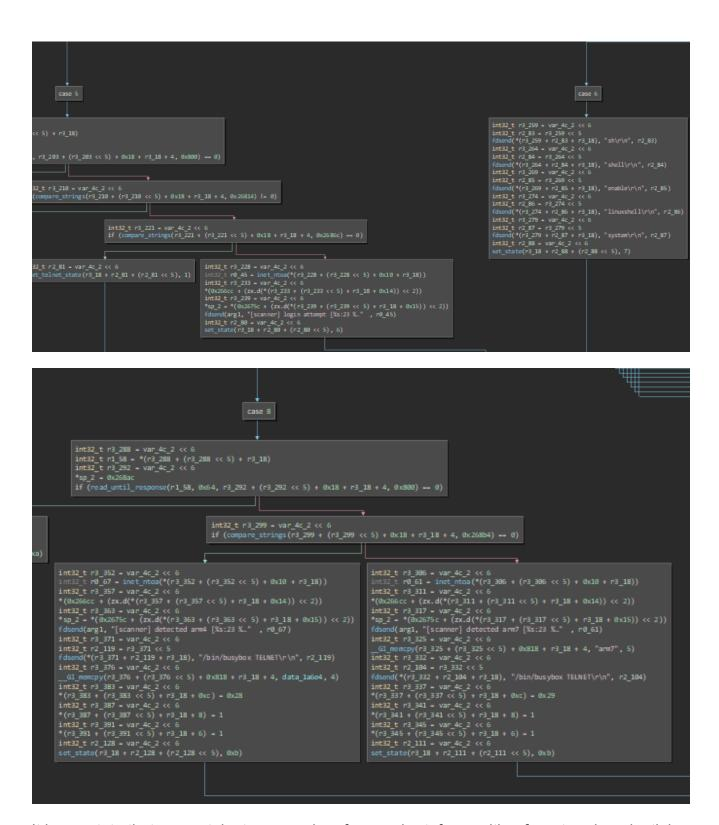
It has a state that runs a telnet scan and performs a bruteforce with a few stored credentials:
