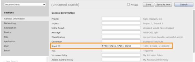
After adjusting the search to cover the applicable time frame, there will be a list of the signatures that fired in the environment during that period. If you click through, you can get details about the systems that are affected and review any packet capture data obtained.
