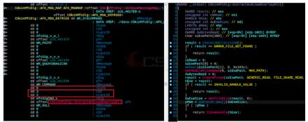
When ExtractAndLoadOverlayDII is called, the hacker will first check if the app has read permission to the Windows\System32 directory and check if the clb.dll file exists. Clb.dll is Windows file - Column ListBox. Then the hacker opens the Exe, reads the Overlay data at offset 0x45800 and xor with 0xA0 to decrypt the PE file is a DLL. It will then manually load this DLL to memory, starting a long series of manually load fileless PE.
