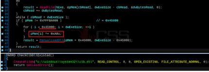
At this ManualLoadDII function, we discovered a hacker programming error. Specifically, Malloc does not have free and wrong code: malloc(sizeof(PE\_LOADER\_INFO)) (16 bytes) to malloc(sizeof(pLdrInfo)) (4 bytes). The PE\_LOADER\_INFO struct that we renamed, including 4 data members, size is 16 bytes.
