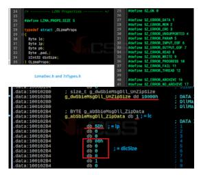
The uncompressed function, the size of the compressed data is passed in minus 4, the size value of the uncompressed data region DWORD immediately preceded the data compressed.
