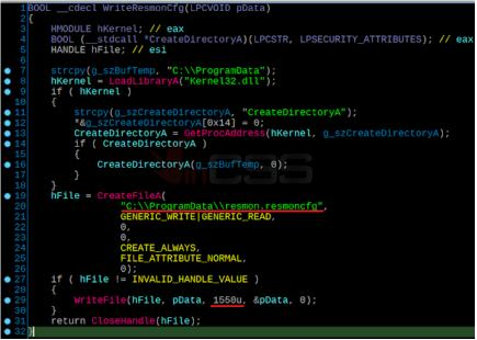
Byte array is the mask for searching is "3F 3E 2F 1E 7F 7E 6F 2E 1F 1E 00 03 3F 3E 2F 4E". File size of resmon.resmoncfg file is 1550 bytes, copy the content from mask offset + 47.
