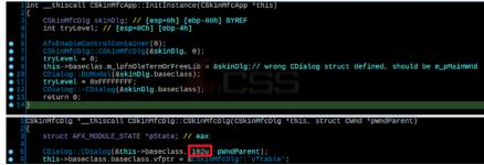
In the OnInitDialog method of CSkinMfcDlg, the hacker has changed the call to the main infection task and added code:
