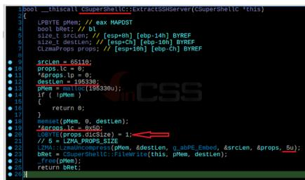
This LZMA algorithm continues to be improved by hackers, so with static dump we could not open, we had to debug and dump it.
