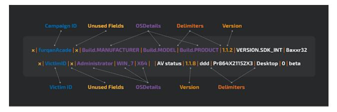
Talos also found some similarities in the beacon creation routine. Both versions have two variables with similar names with the same value, "x," which are then used in the protocol in the same positions. The figure above shows the protocol layout, in the table below you can see each step.
