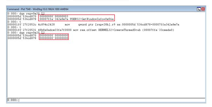
After, CreateThread is placed into RAX and is called. Note CreateThread is actually CreateThreadStub. This is because most former kernel32.dll functions were placed in a DLL called KERNELBASE.DLL. These "stub" functions essentially just redirect execution to the correct KERNELBASE.dll function.
