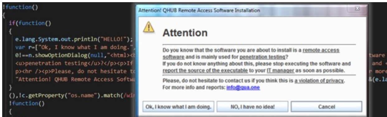
Figure 4: The pop-up User Interface and its code snippet
