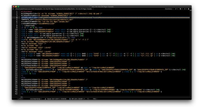
Note line 4, which defines a variable with around 850Kb of base64-encoded data. At line 40, that data is piped through the base64 utility for decoding, dropped in a subfolder in the /tmp directory, given executable permissions via chmod , and then launched as the 2nd stage payload.
