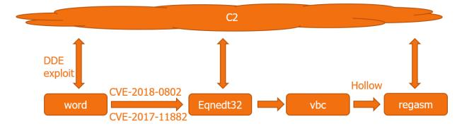
The attached RFQ document is a known macro-less DDE exploit that will download its next stage document from a C2. In order to reduce the risk of detection, the attackers implemented a known <u>technique</u> to avoid the use of "DDE" as part of the text and to delay the download until after protected mode is disabled.
