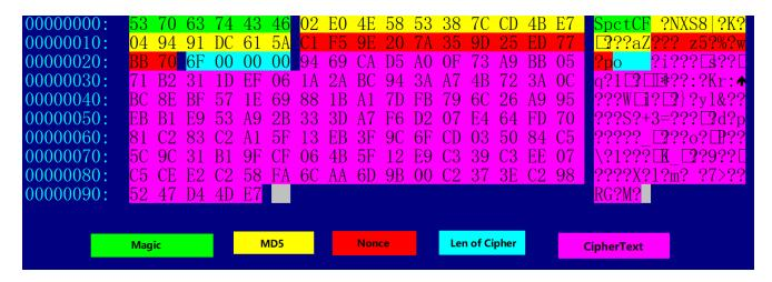
Take the Config in the above figure as an example, the nonce (12 bytes) required for decryption is:
