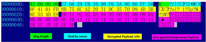
Where Encrypted Payload\_info stores the payload verification, length, ID and other info. [Encrypted?]Compressed Payload is the payload itself, the payload will only be compressed during the key exchange stage, while in all the other stages it gets both encrypted and
