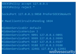
Figure 10. The Tor configuration file used by the latest version of the malware
