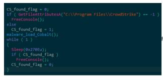
Figure 1: Decompilation showing CrowdStrike specific detection logic
