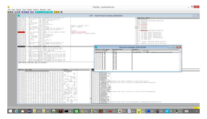
The first two bytes in the structure represents the destination port and we can see that it is 443 in this case.
