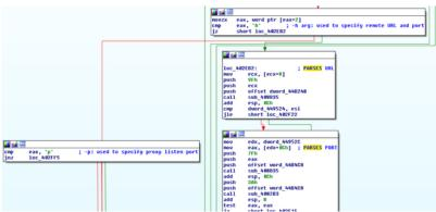
Figure 3 - This structure is utilized to parse the proxy port or remote C2 server from the command line arguments.
