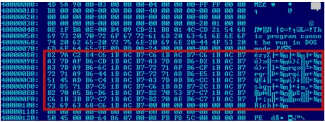
Figure 1: PE binary with Rich Headers highlighted.
