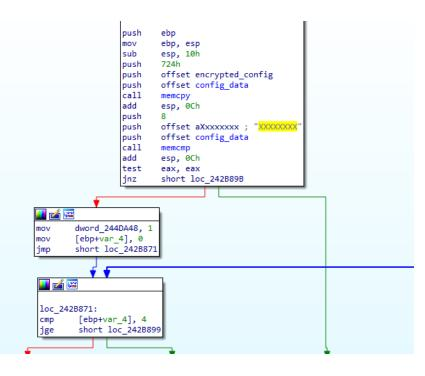
Figure 4: check config data before decryption
