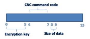
Figure 7: structure of C&C communication header
