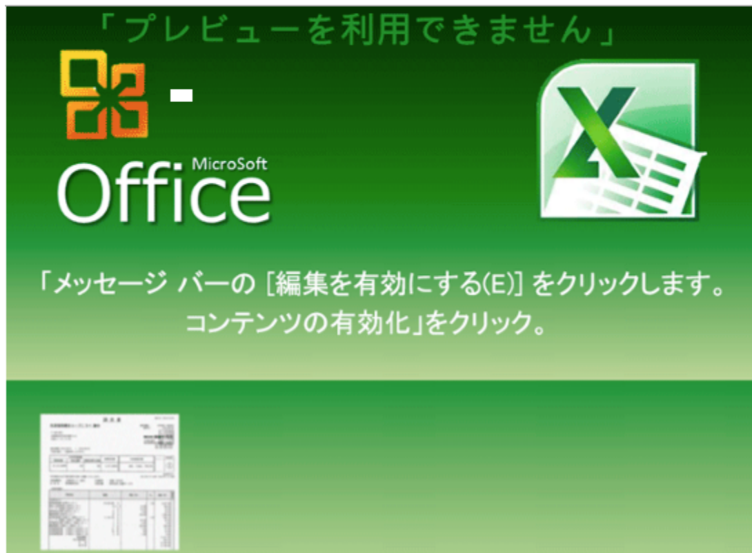
Weaponized Excel document that encourages the user to click on Enable Content .
