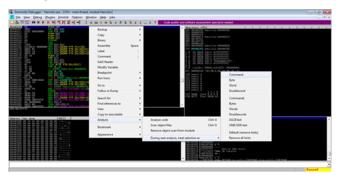
From there, scroll down. You'll notice strings such as "VirtualAlloc" and "\_stricmp" – this section loads different DLLs and imports functions. You can step through this and analyze it, or you can scroll down until you see the last API being imported, which in this case is "memcpy". After a call to GetProcAddress ([EBP-28] here), EAX (memcpy) is moved into [EBP-30]. Put a breakpoint on this and execute the program.
