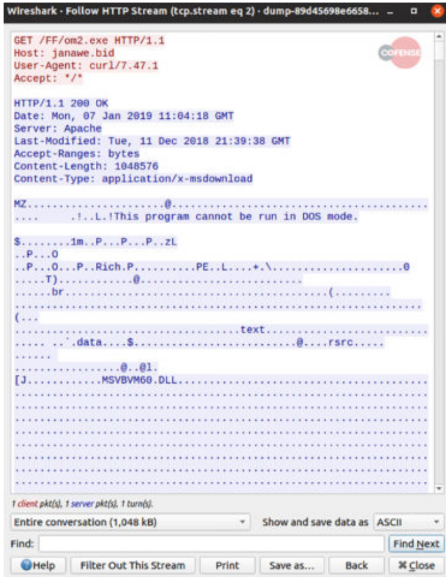
Figure 24: Kutaki uses cURL to download and execute a secondary payload. Note the User-Agent string “curl/7.47.1”.
