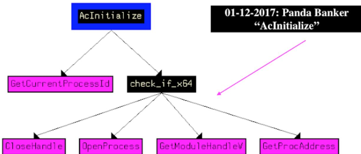
The functions contain check x64 process check via IsWOW64 returning an integer value.
