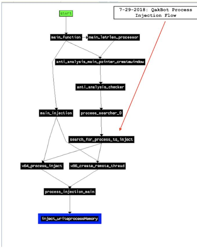
The execution sequence is as follows injecting code into "explorer.exe" in both x86 and x64 variants:
