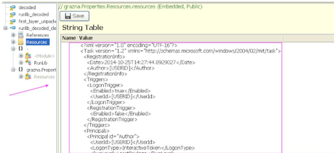
The binary sets up persistence via the task scheduler XML file with its template stored in the resource section. The function is called internally "**okapise.**"
