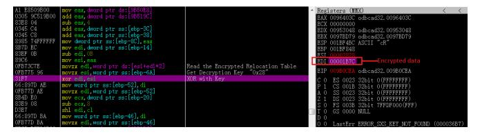
Figure 5: Relocation table being decrypted using a hardcoded XOR key.
