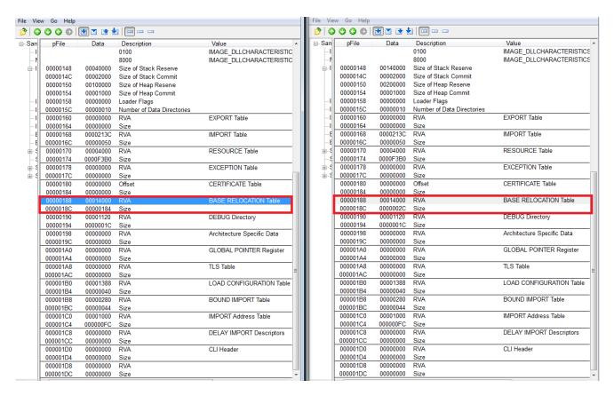
Figure 3: The latest Expiro variant reduces the size of the relocation table.
