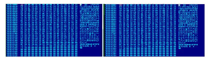
Figure 2: The relocation table contents are not modified by the old Expiro variant.
