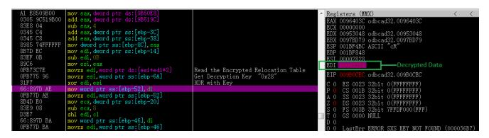
Figure 6: The EDI register now contains decrypted relocation data.
