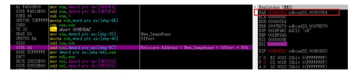
Figure 7: Calculation of the address to be relocated in Expiro's code.
