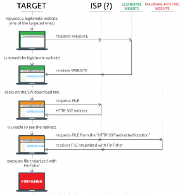
Figure 2: Detailed infection mechanism of latest FinFisher variants
