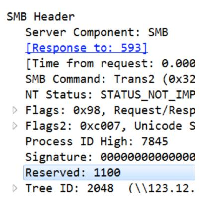
Prior to triggering the code to exploit the system, the "Reserved" field in the SMB header is checked to see if it is set to 0x11.
