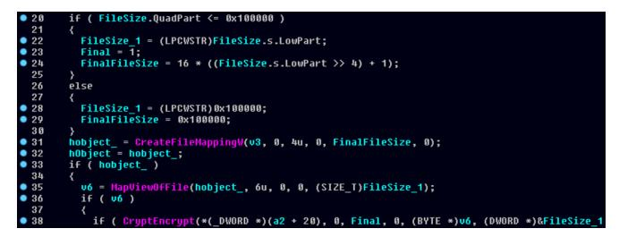
As the above image shows, line 20 compares the file size with 0x100000 (1,048,576 bytes or 1MB). If the file size is greater than 1MB, line 26 declares variables FileSize\_1 and FinalFileSize to be 0x100000. These values are then used in CreateFileMappingW, MapViewOfFile and CryptEncrypt to encode the first 1MB of the file contents. The rest of the file remains untouched.
