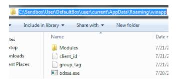
Once everything is copied to the new folder, petya.exe closes and odsxa.exe takes over. odsxa launches SVCHOST.EXE in a suspended state and proceeds to inject data into a new section of the file's memory segment. This is called Process Hollowing and allows the injected code greater freedom in the Windows operating system because it is running under the security context of SVCHOST.EXE.
