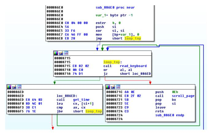
Looking inside the EternalPetya code, we are almost sure that this function was patched post-compilation, rather than recompiled. The first jump, that was supposed to lead to the loop leads directly to the function end:
